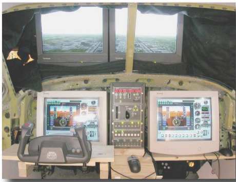
Figure 2. Displays of simulated external view and instrument panel.
