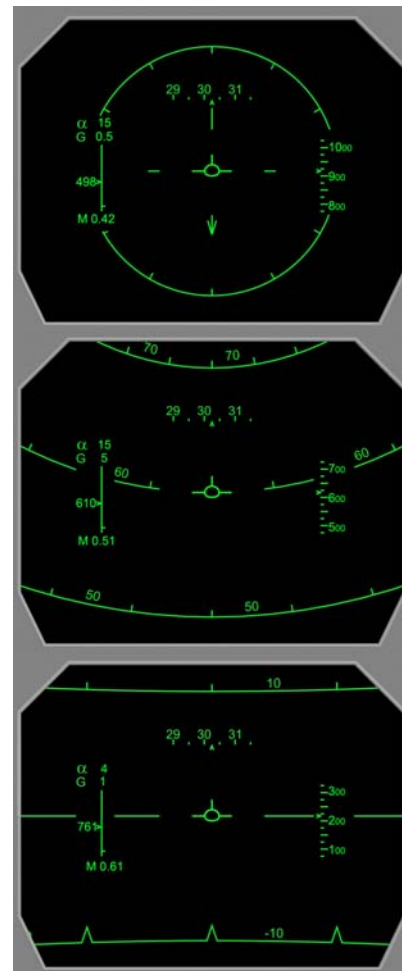
Figure 2. From bottom to top: Pitch attitude of 4° with velocity vector at 0°, 75° pitch-up with velocity vector at 60°, and 75° pitch-up with velocity vector at 90°.
