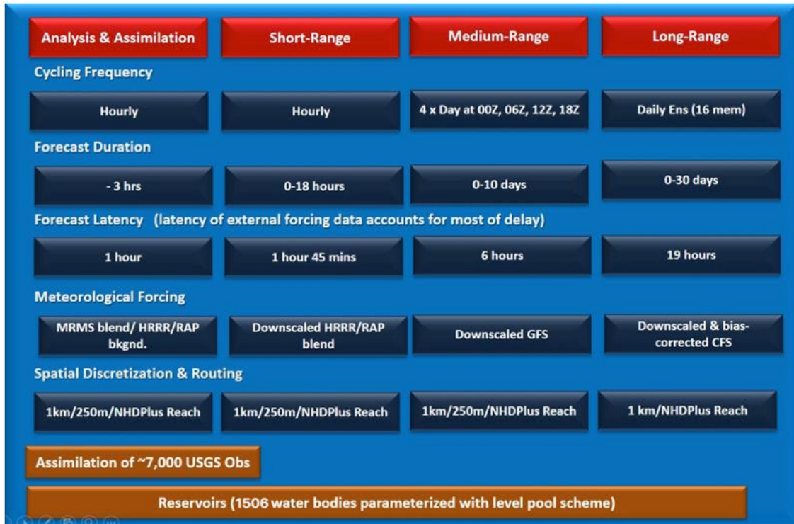
Figure 4-1: Four configurations of the NWM, the data used, and the associated frequencies (adopted from the NWM website at http://water.noaa.gov/about/nwm )
