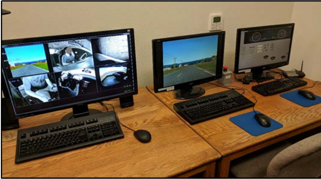
Figure 6.3: Operator workstation for full-scale driving simulator. Monitors are shown displaying SimObserver (left), and the simulated environment (center) or vehicle dashboard (right) as seen in the vehicle
