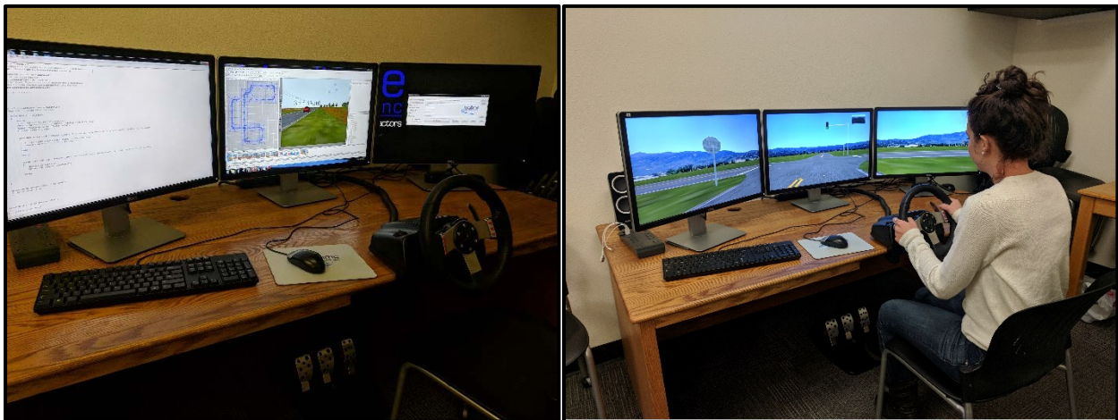
Figure 6.1: Operator workstation for driving simulator. Left: Designing an experiment in the Internet Scene Assembler with Javascript. Right: Researcher evaluating a newly designed environment
