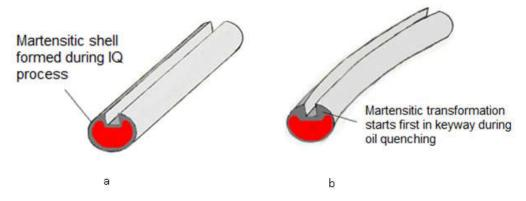
Fig. 3 Martensitic uniform shell formation in keyways during IQ process: *a* – providing minimum distortion due to uniform shell formation during IQ process; *b* – resulting in more distortion due to non-uniform shell formation during oil quenching (Table 1)
