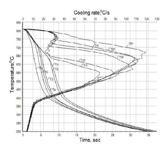
Fig. 8. Cooling curves and cooling rates for solutions of polyisobutylene polymer (PIB 2400) in I – 20A mineral oil at 50°C versus concentration, %wt: 1-0; 2–0.5; 3–1.0; 4-1.5; 5-2.0; 6–3.0 (Logvynenko *et al.* 2016; Kobasko *et al.*, 2016)
