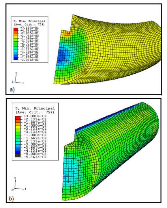
Fig. 2. Minimum principal residual stresses in keyway shaft after quenching in oil (a) and after IQ process (b) according to author (Ferguson, 2013)
