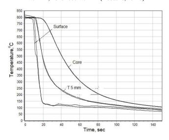
Fig. 7. Cooling curves obtained during quenching cylindrical probe 50x200 мм in 14% water solution of NaCl at 35<sup>o</sup>C: T5 мм is distance 5 mm below surface
