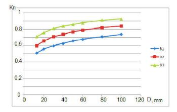
Fig. 6. Effective number Kn versus size of cylinders for different convective heat transfer coefficients: B1 is 750W/ m<sup>2</sup>K; B2 is 1500 W/ m<sup>2</sup>K; B3 is 4000 W/ m<sup>2</sup>K (Kobasko, 2017b)
