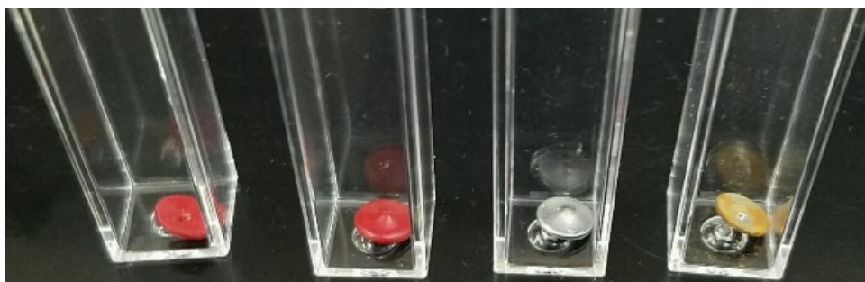
Figure 3. Two metal coupons from a mock sculpture (left) and two unpainted control samples (right).
