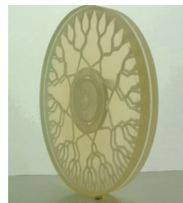
Figure 17. SolidWorks sectional view of dendritic disk, and photographs of a 3D-printed device. Annular plenum and tree-shaped bifurcating channels can be observed. 15
