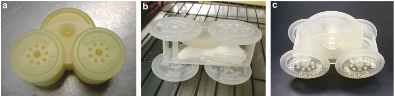
Figure 1. A small push toy car created by a single print on a ProJet 3500 of 3D Systems: (a) out of the printer, (b) melting the support material away, and (c) final functional car produced in a single build with no assembly. The car utilizes a flywheel to store energy, allowing it to travel up to 25 feet (T. Snyder).
