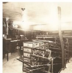
Step 5. The book is taken to a central station in the Bookstacks of the Central Library of the Free Library of Philadelphia where it will begin its automated journey on the conveyor system to the Main Reading Room
