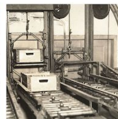
Step 9. The box with the requested book is raised by a dumbwaiter from the first mezzanine level to the Main Reading Room of the Central Library of the Free Library of Philadelphia
