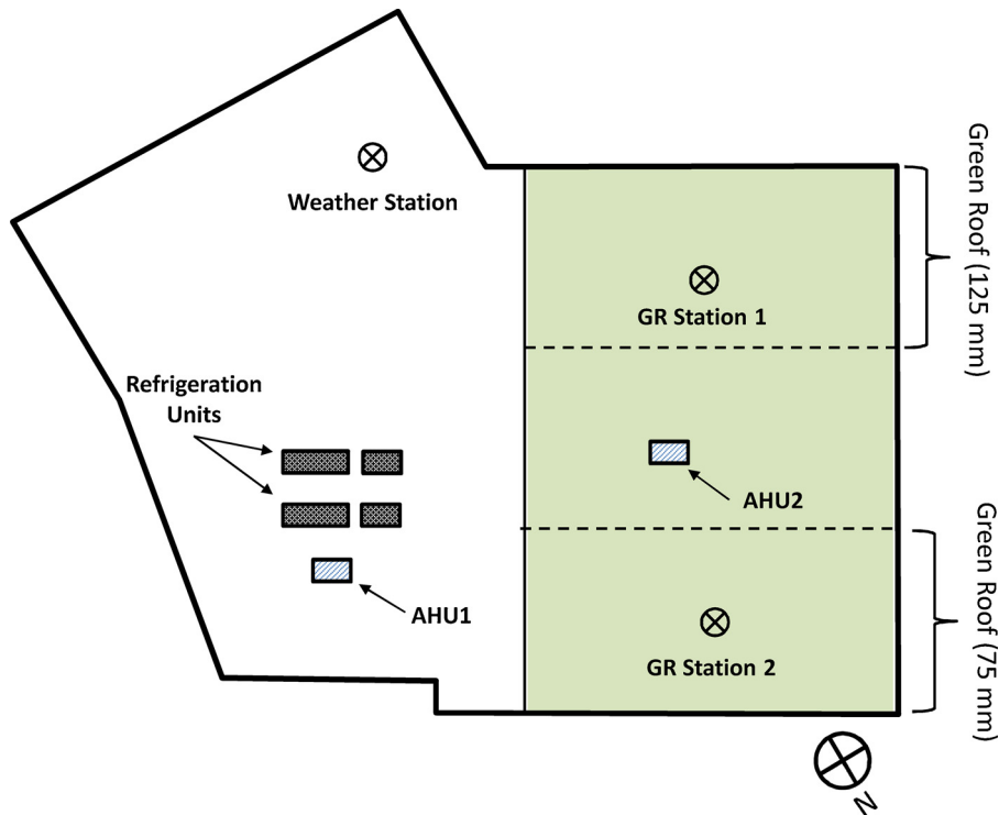
Fig. 1. Layout of the rooftop including the white roof section and the three green roof (GR) sections. The locations of the three weather stations and Air Handling Units (AHU) are marked.
