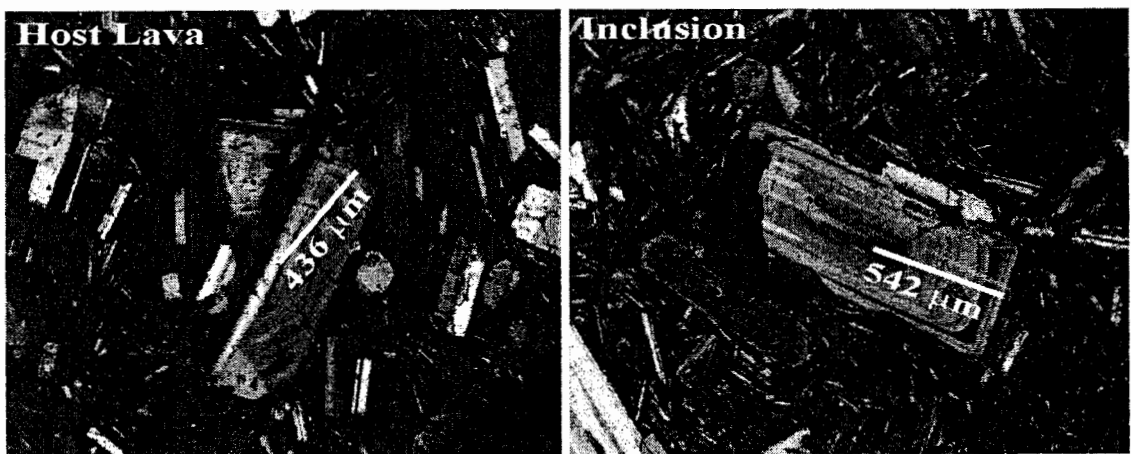
Figure 15 – Traverses conducted by electron microprobe of a representative plagioclase phenocrysts from host lava (left) and inclusion (right) for site 0205. Oscillatory zoning is prevalent. Electron microprobe profiles are shown in Figure 14.
