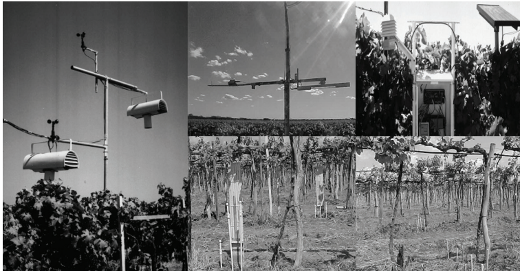
Figure 2. Measurements of gradients of air temperature, vapor pressure and wind speed; incident and reflected shortwave; net radiation; acquisition data system; and soil moisture in Bowen ratio system of wine grape.
