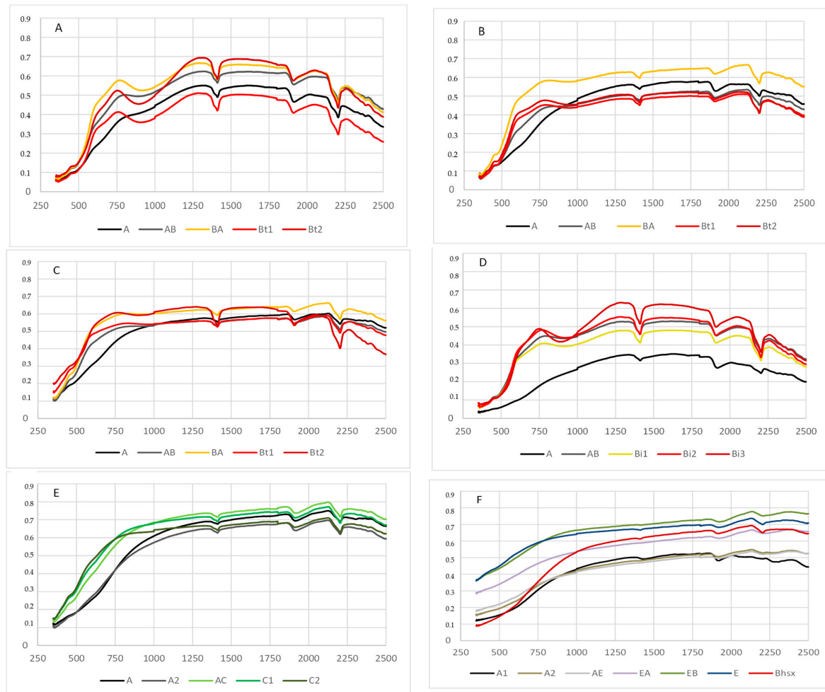
Figure 2. VIS-NIR spectral curves of the horizons of a Red Argisol (A), Yellow Argisol (B), Greyish Argisol (C), Red Cambisol (D), Neosol (E), and Spodosol (F).
