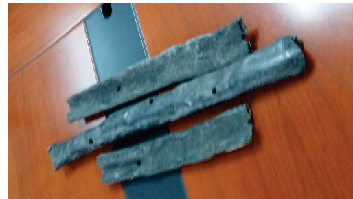
Figure 7 Diagram of pipes with many small holes after actual compression and destruction in boreholes
