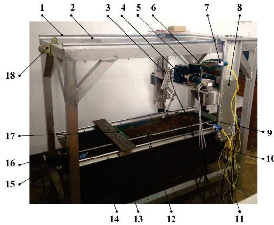
**Figure 9** Soil bin test-bed for single leg: 1 - Slider, 2 - Frame, 3 - Leg brace, 4 - Digital torque and rotational speed sensor, 5 - Coupling, 6 - DC Motor, 7 - Limit Switch 1, 8 - Screw slide module, 9 - Robot leg, 10 - Stepper motor 1, 11 - Limit switch 2, 12 - Ball screw, 13 - Slider, 14 - Soil bin, 15 - Plummer block housing, 16 - Stepper motor 2, 17 - Soil scraper, 18 - Fixed pulley.
