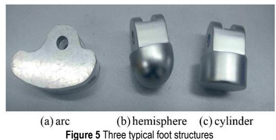
**Figure 5** Three typical foot structures
