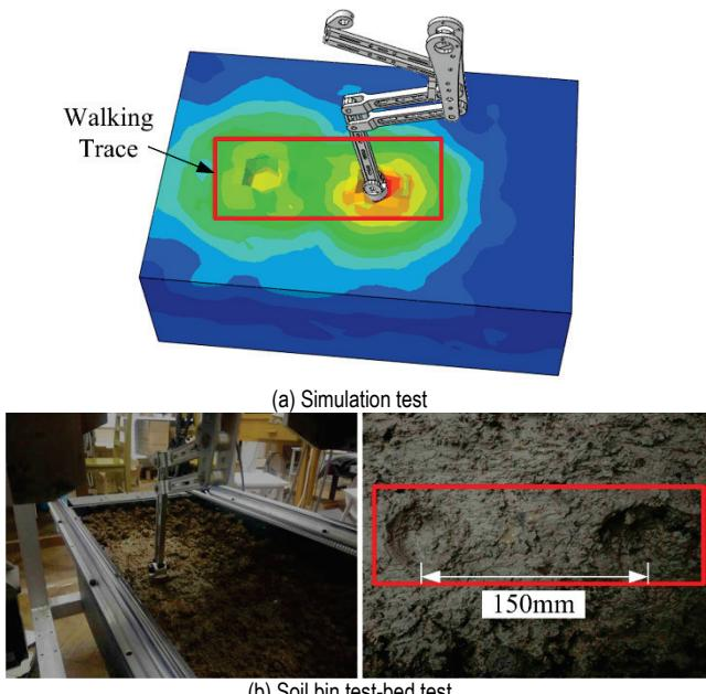
**Figure 10** Interaction between foot and soil
