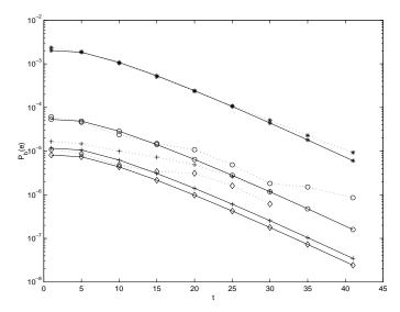
Fig. 5. Residual bit error probability after decoding of the concatenated coding scheme versus the error correction capability t of the BCH(1023,k) outer code, with I = 2 iterations (\*), I = 4 iterations ( $\circ$ ), I = 7 iterations (+) and I = 10 iterations ( $\diamond$ ). The solid curves are related to the performance of the fitted model, whereas the dotted curves show simulation results.
