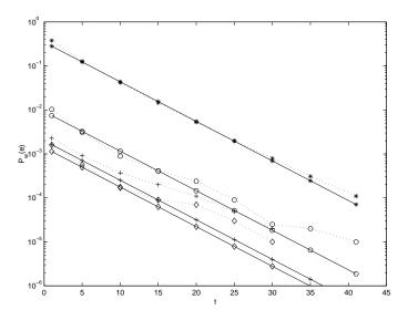
Fig. 6. Residual frame error probability after decoding of the concatenated coding scheme versus the error correction capability t of the BCH(1023,k) outer code, with I = 2 iterations (\*), I = 4 iterations ( $\circ$ ), I = 7 iterations (+) and I = 10 iterations ( $\diamond$ ). The solid curves are related to the performance of the fitted model, whereas the dotted curves show simulation results.
