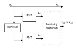
Fig. 2. Turbo encoder block diagram.
