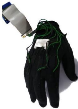
Fig. 3. The Lycra glove system: the glove with 14 flex sensors on the DIP, IP and MCP joint and the IMU device, and the acquisition and transmission box
