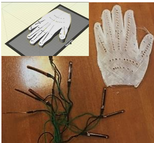
Fig. 1. Flex sensors' wiring (left down) and 3D printed prototype (right up) of the CAD designed glove (left up) [17].
