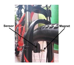
Fig. 2. Magnet on a cycle wheel spoke and sensor mounted on the right suspension fork measure when the wheel makes a spin. [10]
