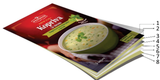
Figure 1 Stand-up pouch Material Layers: 1 - Polyester (PET), 2 - Printing Ink, 3 - Laminate adhesive, 4 - Aluminium (Al), 5 - Laminate adhesive, 6 - Oriented polyamide (OPA), 7 - Laminate adhesive, 8 - Polypropylene (PP)
