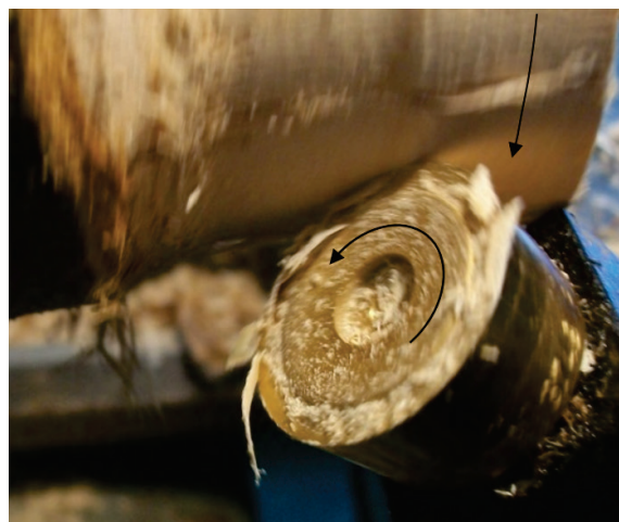
Figure 8 Performance of rotating bowl-shaped tool in turning the wood
