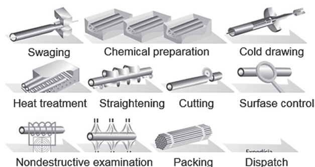
Figure 1 Diagram of production flow of cold-drawn steel tubes
