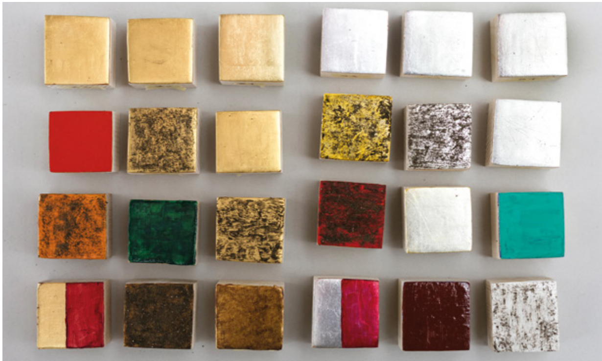
5 Wooden test plates as a simulation of real polychrome and gold-plated artwork (Croatian Conservation Institute Photo Archive, G. Tomljenović, 2017)
