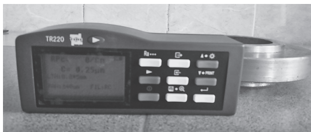
Figure 1 Instrument TR-220 for measuring roughness
