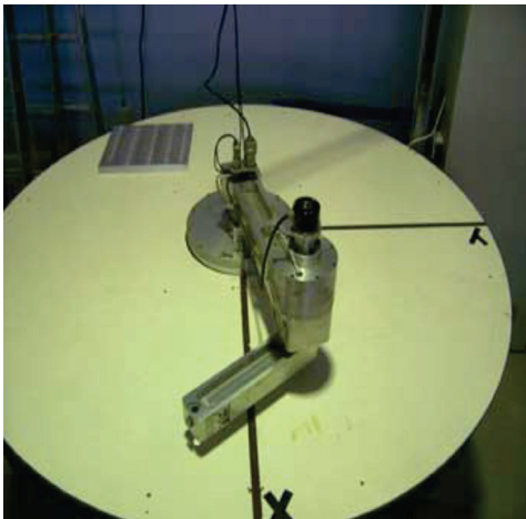
Figure 3 Photo of the IRCCyN SCARA robot
