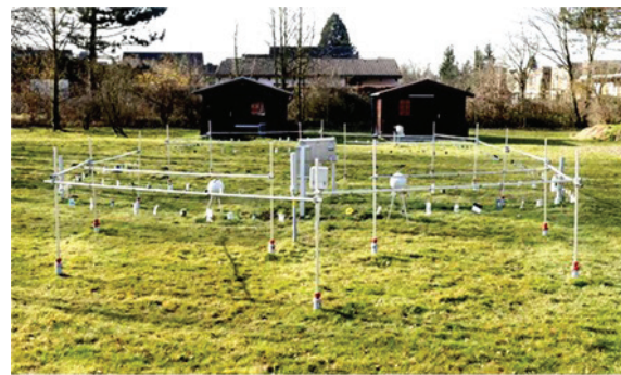
Figure 3 Passive dosimeters exposed at the PTB reference site for environmental radiation. Active reference dosimeters are visible in the middle of the site
