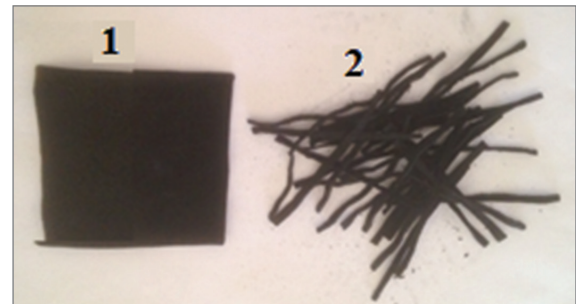
Figure 2. View of two shapes of samples: 1-Square shape [8cm x 8cm], 2-Thin stripes shape
