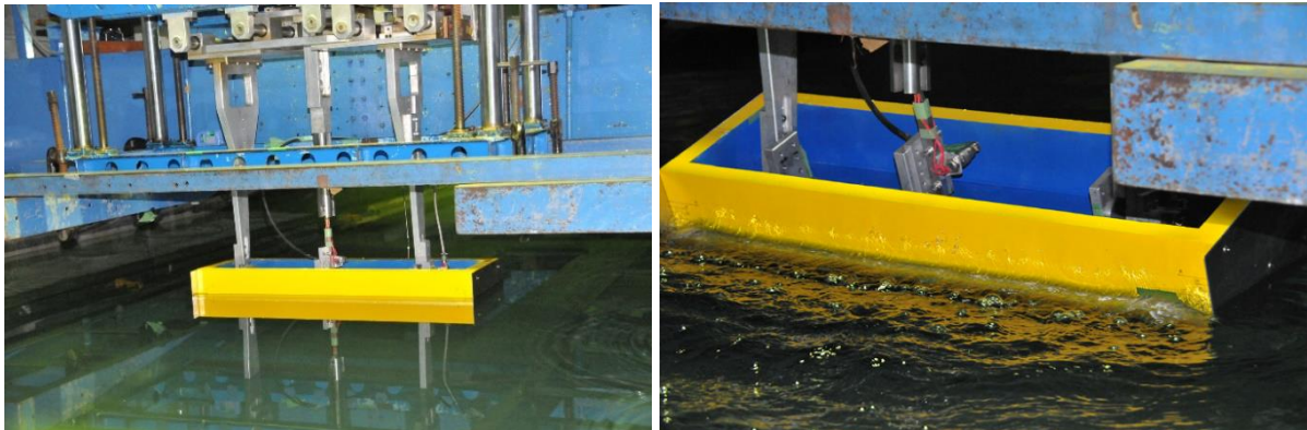
Fig. 1 The 2D midship model attached forced roll mechanism
