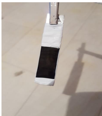
Figure 3. The prochrome plate after using cyclic voltammometry
