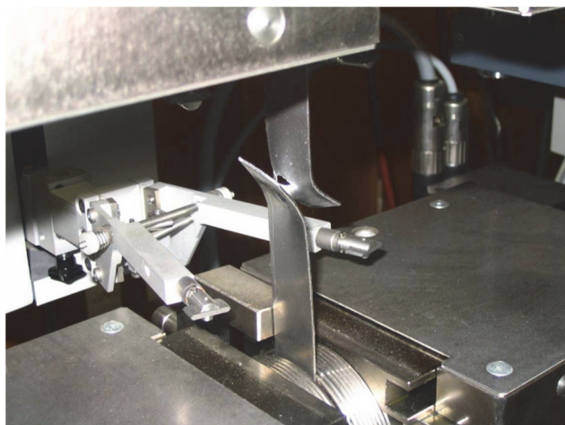
Figure 1 Tension test on Zwick/Roell Z100 testing machine
