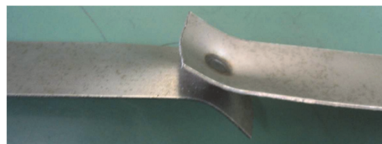
Figure 9 Deformed shape of welded joint obtained in experimental test
