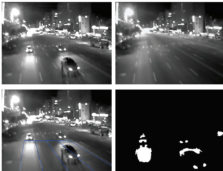
Figure 6 A gray-level input image, the extracted background, region of interest overlapped image, and bright object detected image in the nighttime (from top left to bottom right)
