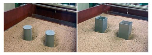
Fig. 11 – Local erosion around two circular and square piers after achieving the equilibrium condition in experiments 6 and 15 on the physical model (see Table 1)
