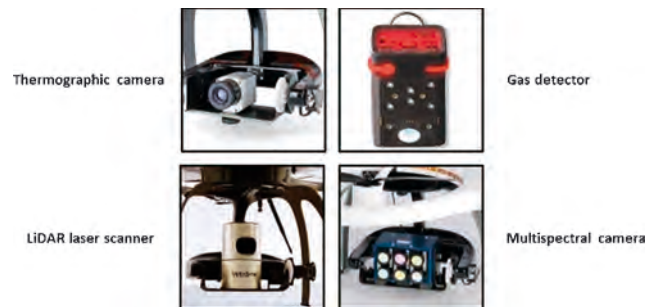
Fig. 2. Various sensors that can be mounted on UAS
