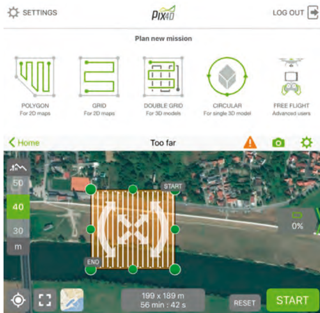
Fig. 7. Application screen for setting up flight mission
