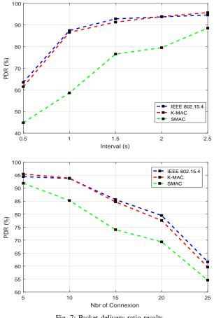
Fig. 7: Packet delivery ratio results
