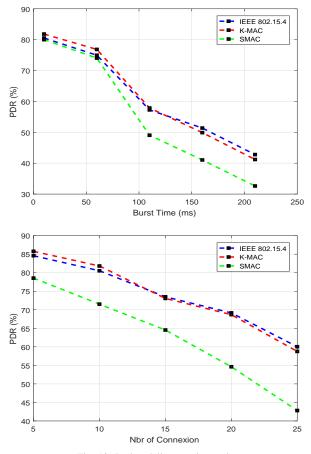
Fig. 10: Packet delivery ratio results
