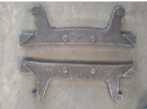
Figure 5. Morphology of grate bar casted by the designed process.
