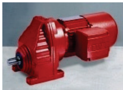
Figure 8 Typical detail of the helical gearmotor with placed ribs in order to make the housing stronger and increase the surface area of housing which transmits the heat with the environment (SEW)
