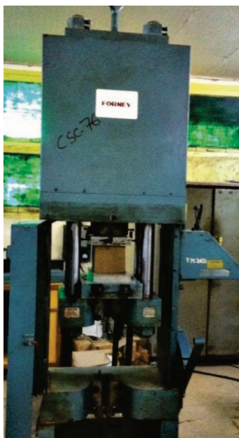
Figure 6 Fired clay cubes are tested in Forney's Universal Testing Machine
