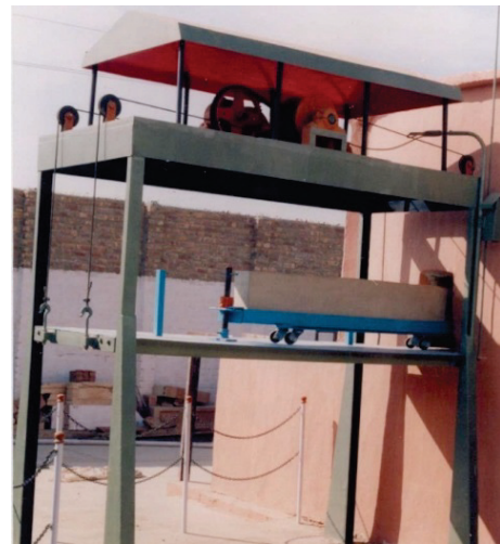
Figure 3 Clay beams being shifted to kiln with the help of platform lift
