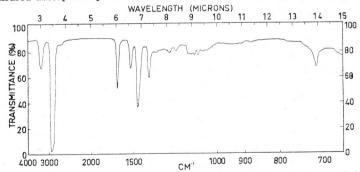
Fig. 3. Infrared absorption spectrum in nujol of synthetic anhydro cerebrin (IIa)
