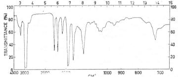
IFig. 2. Infrared absorption spectrum in nujol of analytical diacetyl anhydro cerebrin (IIc)
