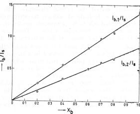
Fig. 1. The calibration-diagram for the quantitative X-ray analysis of borax + amorphous phase mixtures
