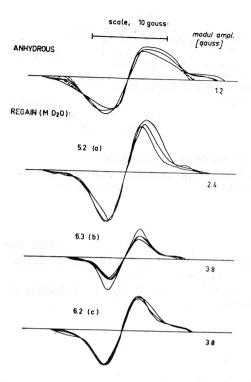
Fig. 3. Proton magnetic resonance spectra (first derivatives) of a completely dehydrated and partially redeuterated samples at room temperature.
