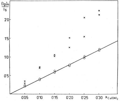
Fig. 2. Calibration graph for quantitative determination of Ca(OH)\_2. o — corrected intensities  $\rm X$  — uncorrected intensities
