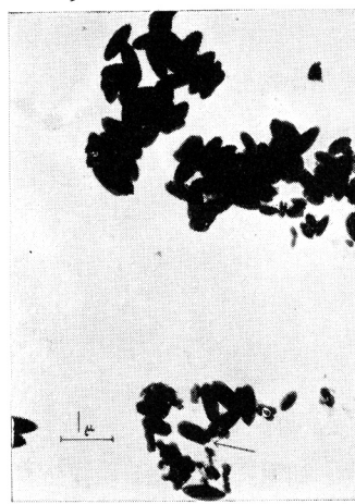
Figs. 1a—e. Electron micrographs of barium sulfate particles formed at several reaction times. a. 40 min; b. 60 min; c. 80 min; d. 100 min; e. 120 min; (concentration of reactants: 4.4 \times 10^{-3} M )
