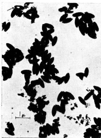
Figs. 1a—e. Electron micrographs of barium sulfate particles formed at several reaction times. a. 40 min; b. 60 min; c. 80 min; d. 100 min; e. 120 min; (concentration of reactants: 4.4 \times 10^{-3} M )
