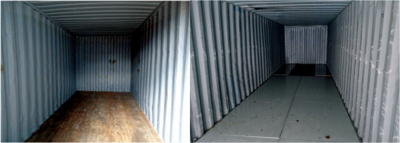
Figure 4 Container before and after the flooring innovation option application
