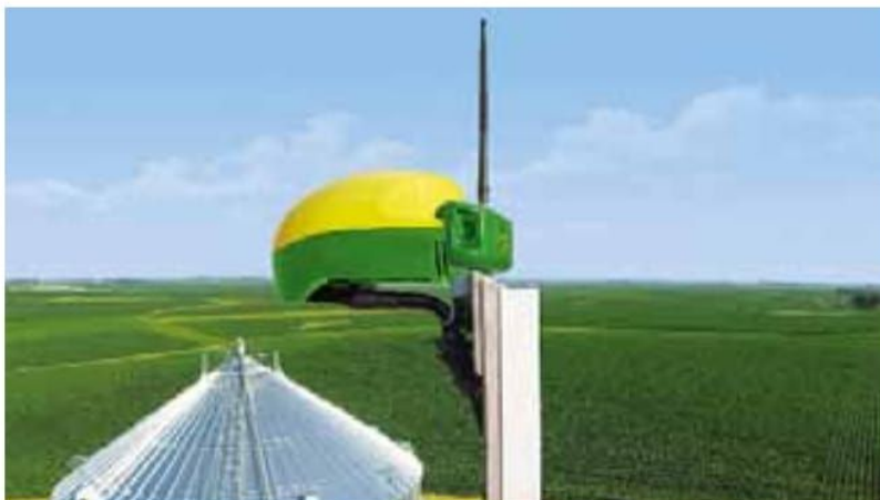
Slika 1. Stacionarna (nepromjenjiva) RTK stanica Figure 1 Stationary (fixed) station RTK
