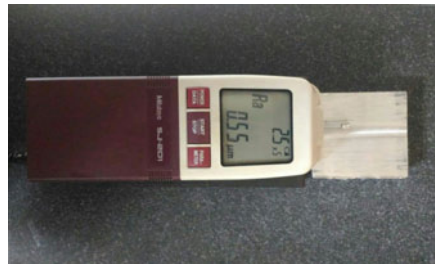
Fig. 1c Surface roughness tester SJ-201
