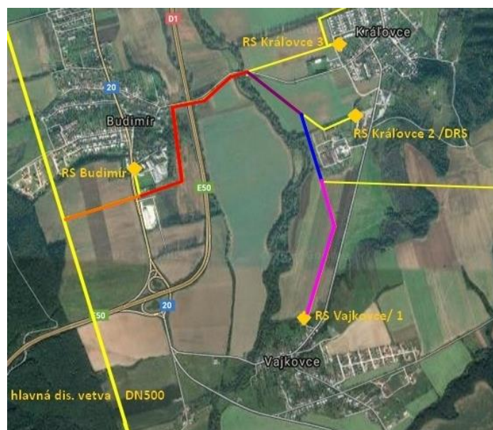
Figure 3. Routing and splitting the gas pipeline into sections (by colours) Slika 3. Usmjeravanje i razdvajanje plinovoda u dijelove (po bojama)
