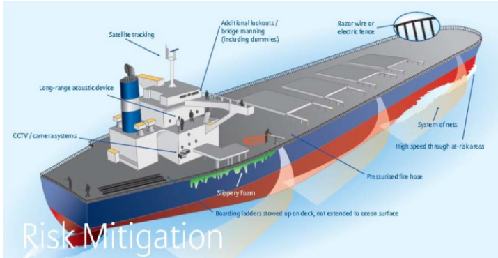
Fig. 3- BMP types of physical protection measures against pirates. Source: Allianz - Piracy: An ancient risk with modern faces, an insurer's perspective from Allianz Global Corporate & Specialty)
