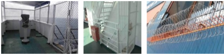
Fig. 2. Physical barriers to protect certain parts of the ship. Source: Private archive
