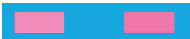
Figure 6 Used sample with the background of 100% RTV and the inner squares of 55% RTV (L) and 65% RTV (R)
