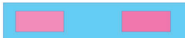
Figure 4 Used sample with the background of 50% RTV and the inner squares of 55% RTV (L) and 65% RTV (R)
