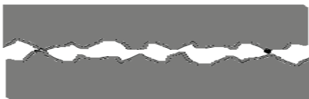
Figure 8 The contact of two apparently smooth surfaces
