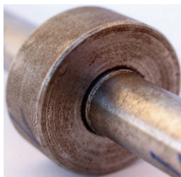
Figure 3 The model of a wheel/axle forced-in joint
