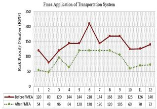
Figure 3 RPN values for before FMEA and after FMEA
