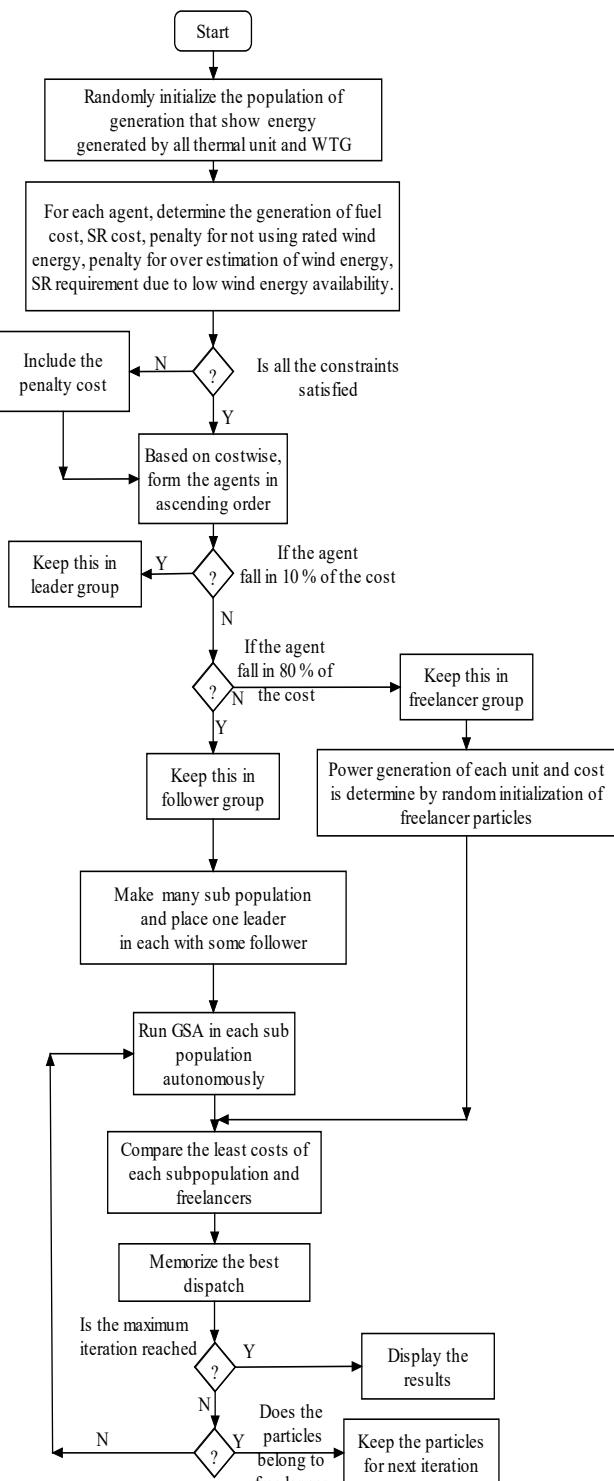
Figure 5 Flowchart for multi objective SDG placement problem using CGSA
