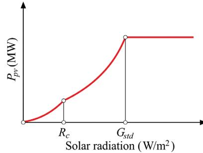
Figure 1 Power curve of Solar Distributed Generation
