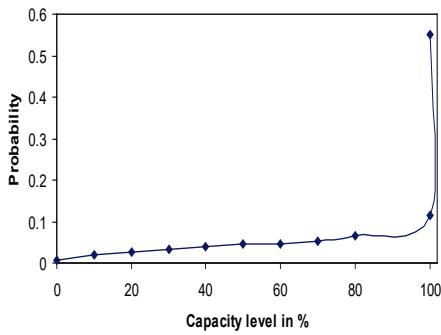
Figure 3 Capacity outage probability profile for SDG unit
