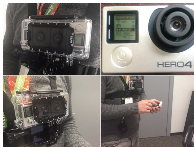
Figure 2 A system of double reverse camera placed on the cameraman's chest
